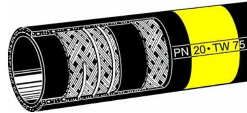
"Yellow Band" smooth bore tank truck hose with kink resistant steel helix for all petroleum based products. Temperature range -30° up to +90° Celsius (temporarily up to 110° C). Electrical conductivity < 10<sup>6</sup> Ohm. - Approved to German military standard VG 95 955 type S. Complies with EN 12115 and EN 1361 E.
